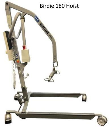
This hoist has an electrically operated arm controlled by a remote and manual push levers for adjusting the leg width.
